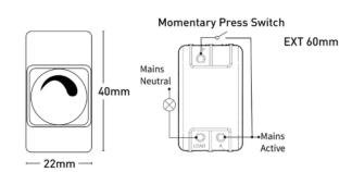
Note: A momentary press switch returns to the open position when released. If an external switch cannot be installed, leave the 'P' control terminal unconnected.
