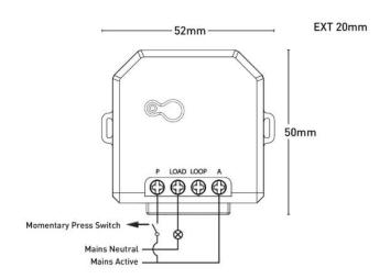
Note : A momentary press switch returns to the open position when released. If an external switch cannot be installed, leave the 'P' control terminal unconnected.
