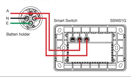
**Smart Switches:** Multi way wiring configuration for non-smart lights. A two way scenario is shown below. Multi way switching is created through the automation section of the Mercator Ikuü app. When using Zigbee switches, only active is required [not a neutral].
